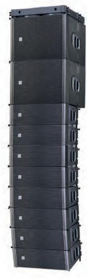
V8 line array speaker is a 2 way system, supplying a frequency scope of 65Hz-20KHz, the design of the cabinets produce a smooth frequency and phase response. Two 44mm tweeter compression units and two 8" bass units form a middle /high frequency system, which decreases greatly the cabinet weight, and supplies a high SPL/volume ratio.
